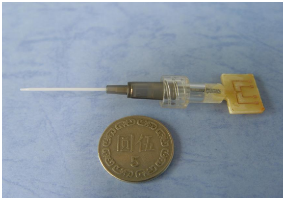
Fig. 4 the catheter-based sensing module
