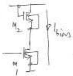
$$\frac{v_{out}}{v_{in}} = - \frac{g_{m1}}{g_{m2}} = - \frac{\sqrt{I_{bias} \mu C_{ox} \frac{W_1}{L_1}}}{\sqrt{I_{bias} \mu C_{ox} \frac{W_2}{L_2}}}$$
