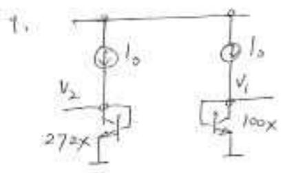
$$V_{out} = V_1 - V_2 = V_T \ln \frac{I_0}{I_s \cdot 100x} - V_T \ln \frac{I_0}{I_s \cdot 272x}$$
